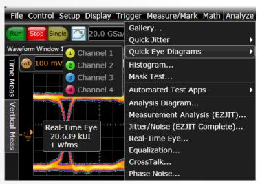
Jitter tests and eye diagrams can be set up automatically with one click in the Analyze menu. An eye diagram on a Tektronix 5 or 6 Series may take up to 14 steps within four different menus.
