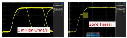
The Tek 4 Series (using FastAcq) can also capture this event, but without the special FastAcq mode the Tek 4 Series fail to show this waveform anomaly. Although FastAcq is fast enough to reveal the information, once the user selects Visual Trigger to isolate the waveform, the Tek scope reverts to a normal acquisition mode with 22 waveforms per second update rate.
